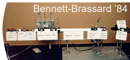
Original Quantum Cryptographic Apparatus built in 1989 transmitted information secretly over a distance of about 30 cm.
