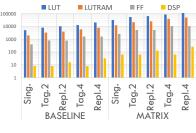
The resource utilization of the multithread accelerators stands in between the single-thread ones and the corresponding set of replicas.
