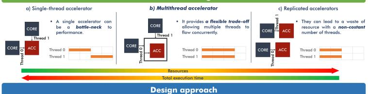
The proposed **model-based approach\*** allows, starting from the single-thread **dataflow specification** of an application and **without** explicit need of **data synchronization**, to design a corresponding multithread hardware
